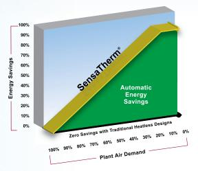
The optional SensaTherm energy management system automatically matches purge air requirements to real time load on the dryer. When operating at reduced capacity, the on-line drying tower remains active until the full drying capacity of the desiccant material is utilized. Each tower is precisely controlled to manage drying times to reduce purge air consumption.
